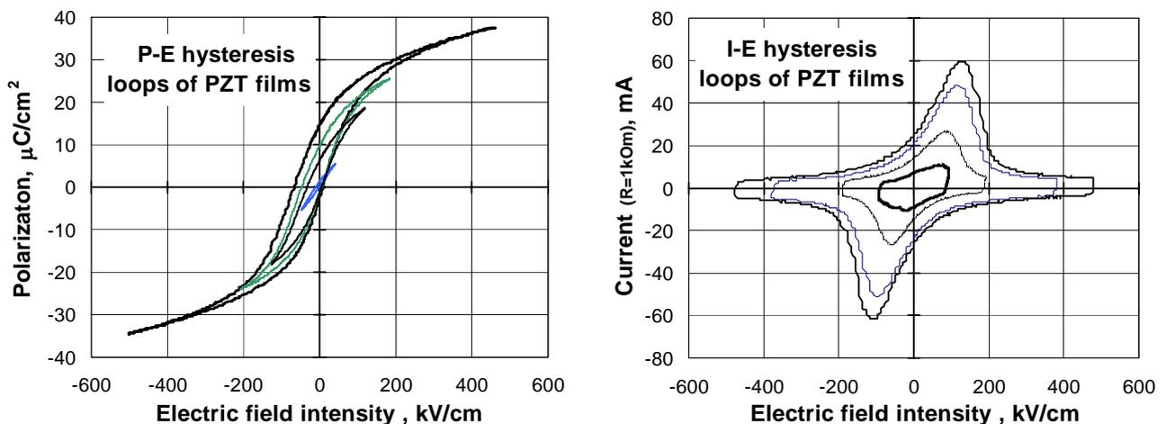
Figure 1. Hysteresis loops: obtained by reference capacitor (the Sawyer-Tower method) and obtained by
