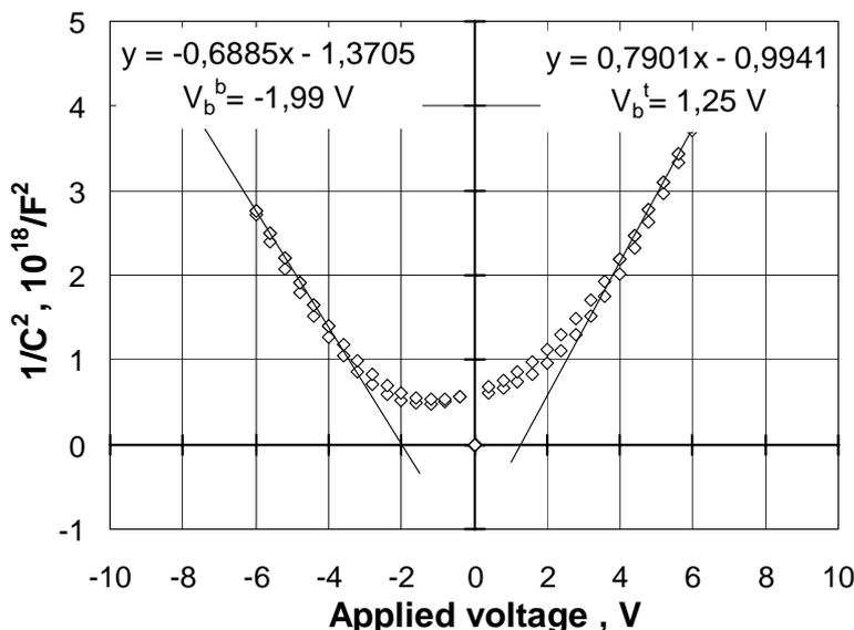
**Figure 4.** C-V characteristics of Pt/PT/Pt/SiO<sub>2</sub>/Si structure and plot of  $(1/C)^2$  vs. V. Solid lines denote the results of linear fitting for the high field regions (magnitudes of interface states density are in region
