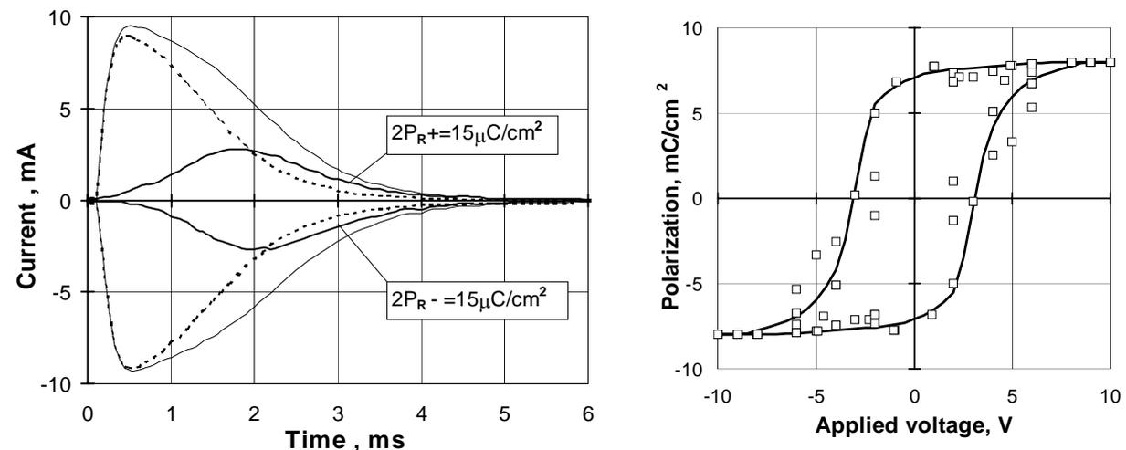
**Figure 3.** Remanent polarization hysteresis obtained from loops the pulse current of polarization switching
