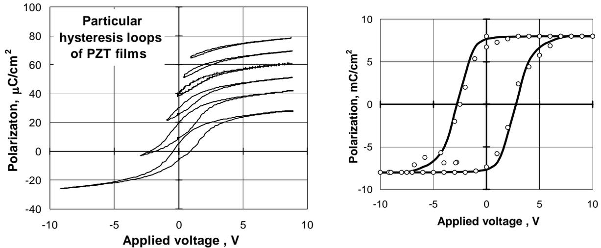
**Figure 2.** Remanent polarization hysteresis obtained from measurements of nonsymmetric hysteresis loops
